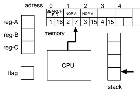
Figure 1: Structure of the virtual CPU in the network-type assembly model.
