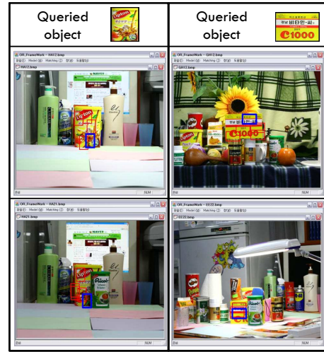
Figure 4: Results of object recognition. The matched candidate regions in input images are outlined
