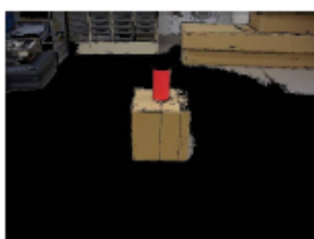
Fig. 13 Floor surface removed (Experiment 1)
