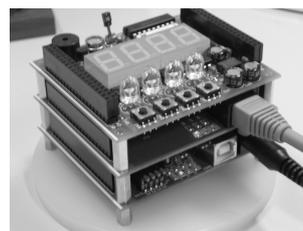
Figure 1: Photo of a Stacked Micro Cube
