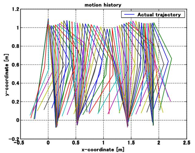
Figure 7: The simulated walking gait of bipedal using two-rank model in Fig. 6
