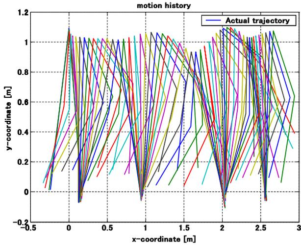
Figure 5: The simulated walking gait of bipedal using one-rank model in Fig. 4
