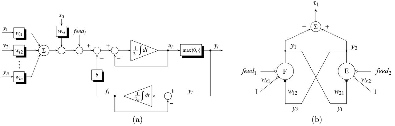
Figure 1: (a) General Matsuoka neuron model; (b) One oscillator consisting of an extensor and a flexor
