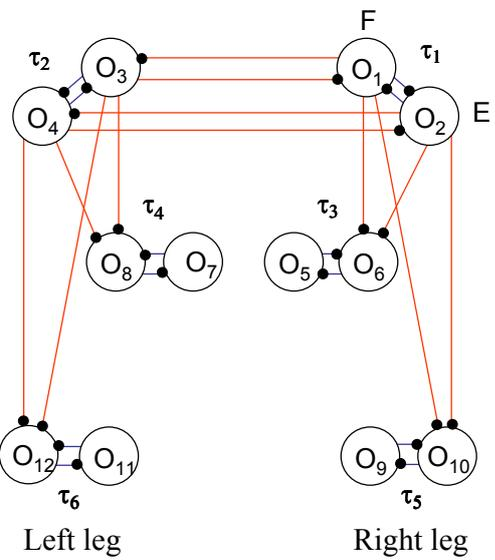
Figure 4: One-rank CPG network of biped model
