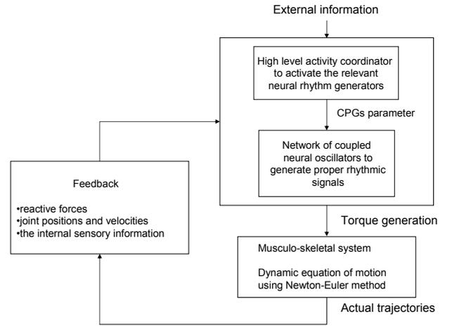
Figure 2: The general control strategy for the bipedal robot
