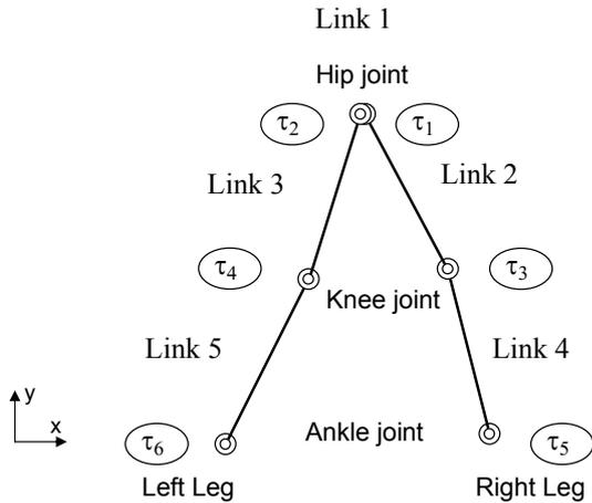
Figure 3: Five link model for a biped locomotion
