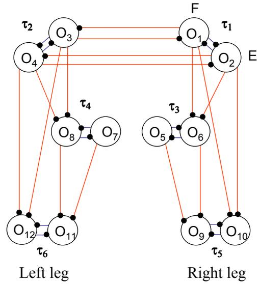
Figure 6: Two-rank CPG network for a biped locomotion
