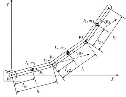
Figure 1: Model of three-link underactuated manipulator
