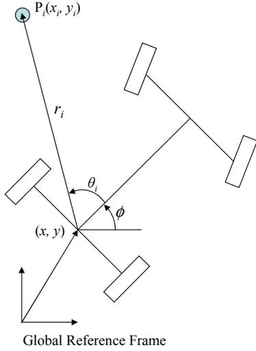
Figure 1: Vehicle and observation kinematics
