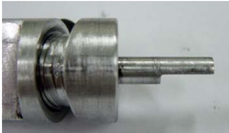
Fig. 10: Frictional wears of piston
