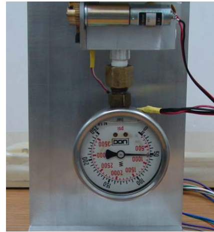
Fig. 8: Pressure value of 50kg/cm 2 measured by manometer
