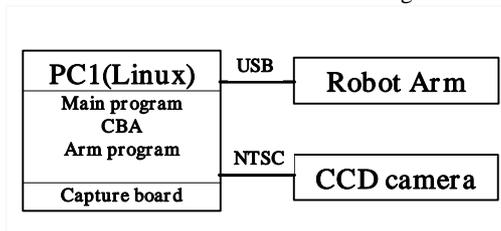
Fig. 2-3 System structure of the robotic arm
