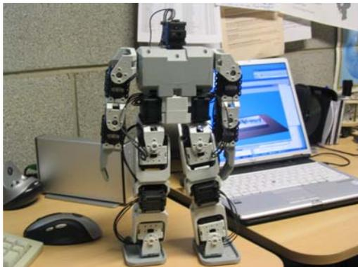
**Figure 6. The Bioloid humanoid robot**
