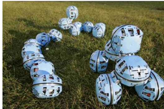
Figure 1. ATRON modules for self-reconfigurable robotics.
