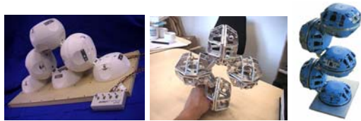
Figure 2. The first, second, and third (final) hardware prototype of the ATRON modules.
