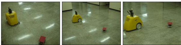
Fig. 11. Capturing operation along the single-curvature trajectory
