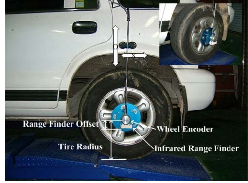
Fig.3 Implementation of wheel encoder and infrared range finder sensor
