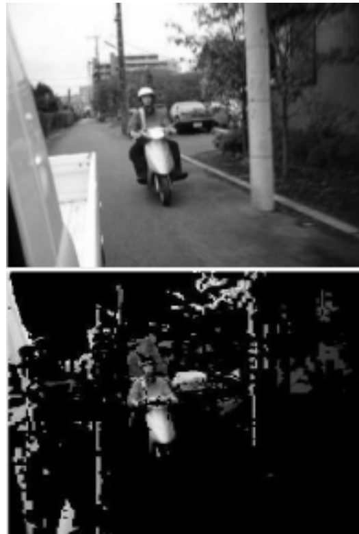
Fig. 2. Original Image (upper) and Conversion Image by HSV color space method (below)
