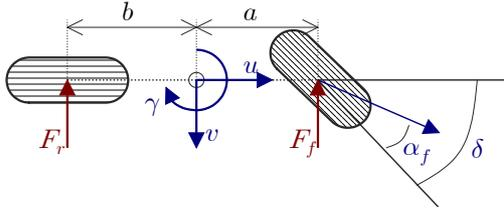
Fig. 1. Coordinate of the single-track model
