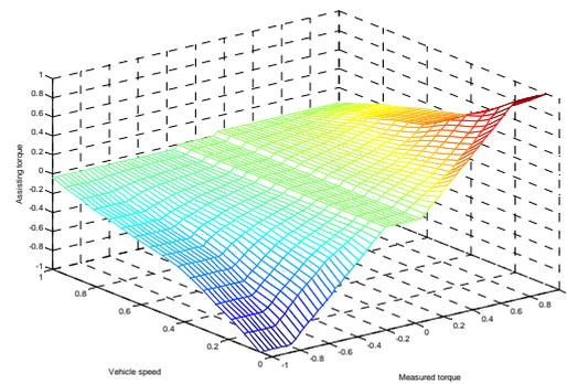
Fig. 3. Normalized control surface
