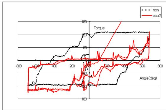
Fig. 4. Plot of steering angle vs. steering torque ( $u = 0$  m/s)
