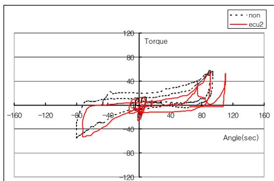
Fig. 6. Plot of steering angle vs. steering torque ( $u = 16.6$  m/s)
