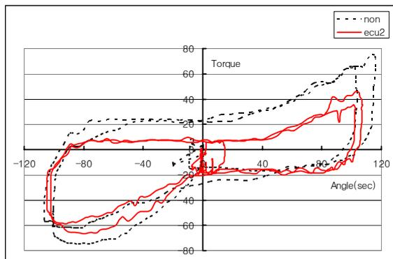
Fig. 5. Plot of steering angle vs. steering torque ( $u = 11.1$  m/s)
