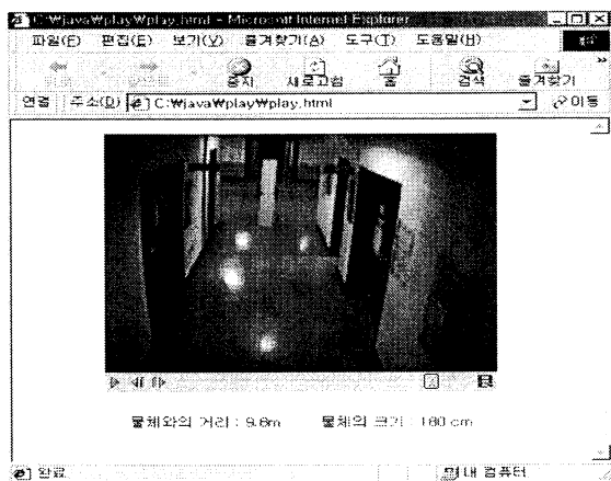
Fig. 4 Measurement of the distance from the camera and the height of an object
