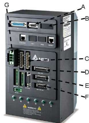
Fig. 3. The PLC-based controller(ASDA-SM)
