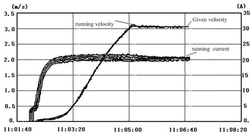
Fig.3 System speed and power curve of actual control
