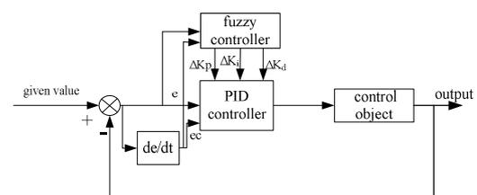
Fig.2 The fuzzy self-tuning PID principle diagram
