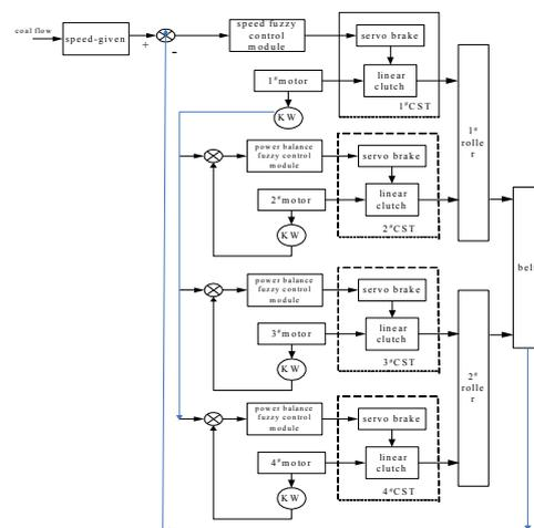
Fig.1 Belt speed and motor power balance control principle
