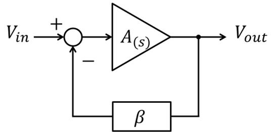
Fig.2. Block Diagram of Voltage Feedback
