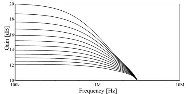
Fig.8. Frequency Response of Conventional IA
