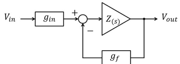
Fig.4. Block Diagram of Current Feedback
