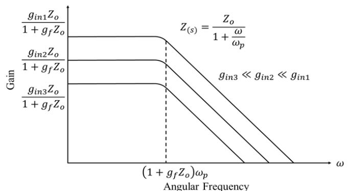
Fig.5. Frequency Response of Current Feedback
