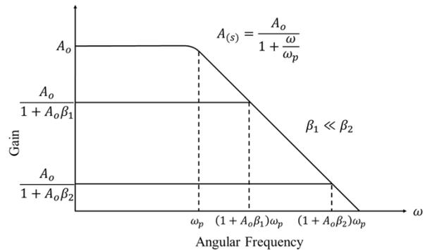
Fig.3. Frequency Response of Voltage Feedback
