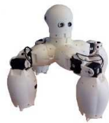
Fig. 1. The robot Fable. An example of a modular configuration comprising four actuated modules and a head module endowed with ultrasound sensors.
